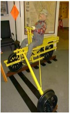
ance. The car is powered by both hand and foot levers. He soon formed the Sheffield Velocipede Car Company and produced about 4,000 cars. The velocipede was used throughout the nation and Europe for railroad signal inspection and maintenance. This particular handcar was used locally in San Luis Obispo on Southern Pacific rails in the early 1900s."
