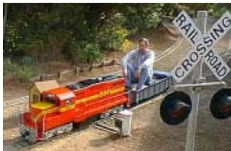
saying is, "This is pretty cool!" This No. 1801 is 1.6" to the foot and is powered by a V-twin, 16-horsepower gasoline engine that runs on regular gas. The engine runs a hydraulic pump which in turn runs hydraulic motors on each truck that drive each axle by chain and sprocket. This No. 1801 will be at SMVRHM's Choo Chew Saturday on May 17 (see page 1 article). Hop on board! 🐞
